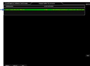
Select [UPDT] from the 2. ADVANCED SV Network menu in Calibration to load new software in all the Dynon remote components.
