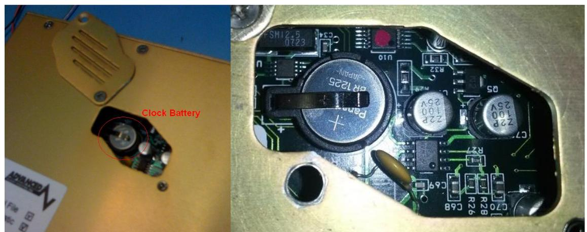
4. Tape your needle nose pliers as shown below. Place some paper around the battery in case the battery tries to fall deep into the unit.
