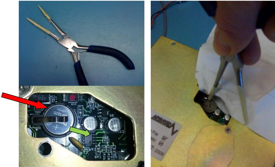
5. The red arrow indicates the location of the notch to push the battery from. This allows the battery to slide in the direction of the green arrow toward the silver can.
